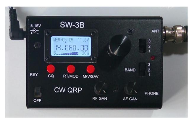
SW-3B is an ultra-small, ultra-lightweight three-band CW QRPtransceiver that consumes less than 40mA when receiving. It is ideal for portable use, field day and SOTA.
