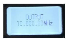
At this time, use the frequency counter to detect the frequency of the TEST point on the PCB board (near the power socket), turn the large knob to adjust the frequency to the frequency counter display 10.000.00MHz, then press the M/V/SAV button to exit.
