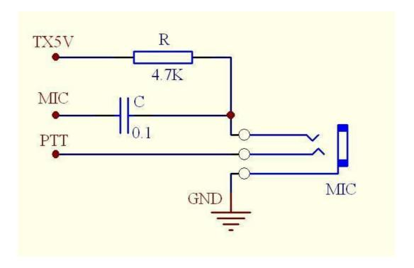
The TX5V, PTT, MIC and GND pads have been reserved on the PCB board, as long as the wires are connected to the corresponding pads as shown in the figure. The mounting hole of the stereo headphone socket should be opened in the appropriate position on the back panel.
