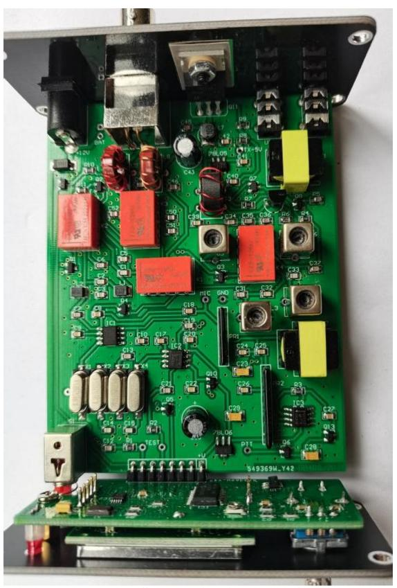
Solder the control board and cut off the excess pin section to install the front panel. The photo of the installed kit is as follows:
