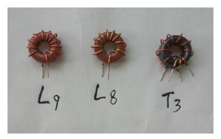
The inductor L8 is wound with a yellow enamel wire 10 turns, and the inductor L9 is wound with a red enamel 12 turns, see photo.
