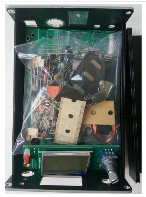
The kit consists of two PCBs, one for the control board and the other for the mainboard. All components on the control board have been installed and tested. There are two integrated circuits and four crystals on the main board are patch components, and the rest are common leaded components. It is easy to install. There are only four inductors to be adjusted in the kit. It can be worked as long as there is no error in the component soldering, and no components issues.
